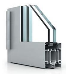
This aluminium door in modular set-up fulfils the requirements of class El30 and/or class T30/F30 for single and double-leaf doors without the need for fire protection inserts. Simply by adding these, class El60 and/or T60/F60 are achieved. A full range of fanlight or fixed top or lateral glazings assure a comprehensive application range.
