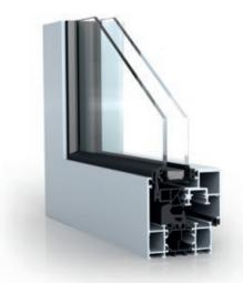
The option "Concealed Sash" in the aluminium window system WICLINE evo features a special glazing bead fixed directly in the thermal break zone. As a result the system achieves an extremely slim frame elevation, superior thermal insulation values and a sleek profile design from outside. The improved ratio between frame and glazing surfaces leads to very good  $\rm U_w$  values, increased light transmissions and panoramic views.
