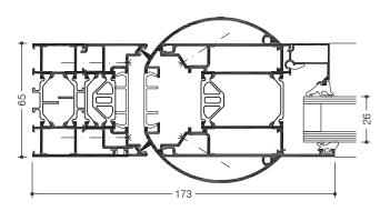
With round profile, fulfils also the finger protection requirements
