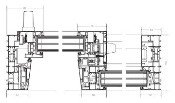
Horizontal section 1 sliding sash + fixed light
