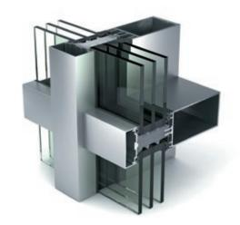
Passive house does not require an active heating system and therefore relies heavily on the thermal insulation and air-tightness of the façade. Based on the standard series, WICTEC 50HI is certified for aluminium/glass façades suitable for passive houses at minimal additional cost. The thermal insulation exceeds the benchmark requirements of passive-house, with a  $\rm U_{\rm f}$  value of 0.65 W/(m²K) thanks to easy-to-install special thermal break profiles in combination with triple glazing.
