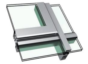
The quality requirements for ventilation sashes are particularly high for those installed in the roof. WICTEC 50 meets these requirements and delivers a delicate appearance with minimal offset of the glass level. Minimised profile widths, concealed hinges with 90° opening angle and the option of large sash formats offer extensive freedom of design. Thanks to the large ventilation cross sections, the WICTEC 50 skylight is also ideal for use as natural smoke and heat exhaust ventilators.
