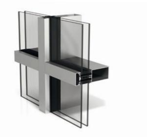
WICTEC 50 is the basic version of the stick system curtain wall, with an extra-narrow face width of 50 mm, inside and outside. The unique flexibility is demonstrated by the various system variants and enhancement options, all of which are feasible with minor additions to the system and without compromising on appearance.
