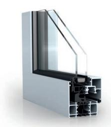
The option "Concealed Sash" in the aluminium window system WICLINE evo features a special glazing bead fixed directly in the thermal break zone. As a result the system achieves an extremely slim frame elevation, superior thermal insulation values and a groove-free profile design from outside. The improved ratio between frame and glazing surfaces leads to very good  $\mathbf{U}_{\mathbf{w}}$  values, increased light transmissions and panoramic views.
